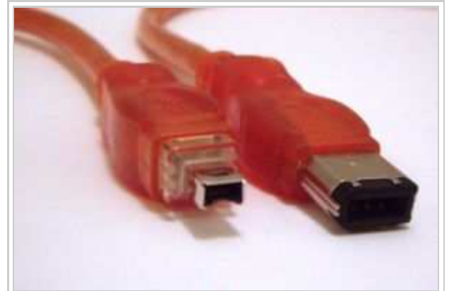
4-pin (left) and 6-pin (right) FireWire connectors
