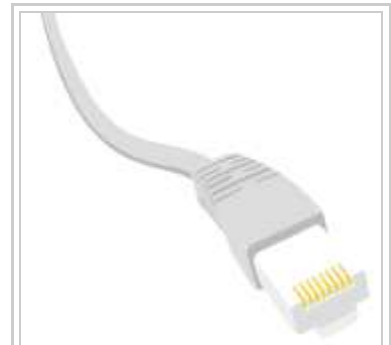
The alternative ethernet-style cabling used by 1394c
