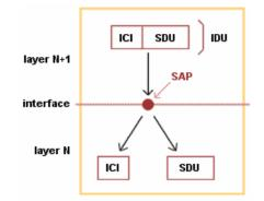
The SDU is the data that 2 peer entities exchange, but it is also what the layer N+1 of the sender gives to the layer N. The control information is used to help the lower layer. It is for example the number of bytes contained in the SDU (this can be used in the function that controls data integrity).
