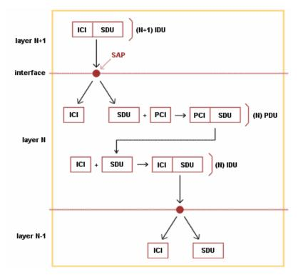
Finally, all messages fit together. This mechanism is often described as a **wrapping** mechanism.
